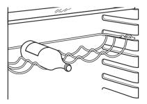
To do this pull the bottle rack forward until it can be tilted upwards, then slide the front support into the next level up.
